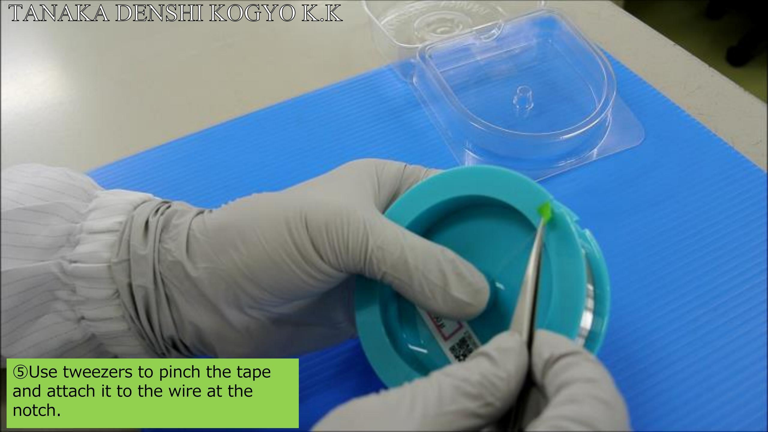
⑤Use tweezers to pinch the tape and attach it to the wire at the notch.
