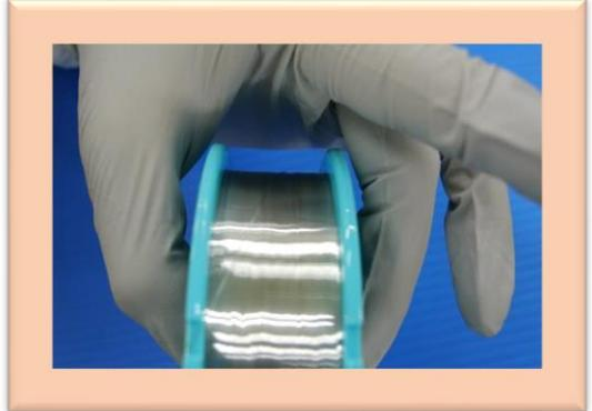
② Hold the center of the spool and pull the wire to remove any loose parts.
