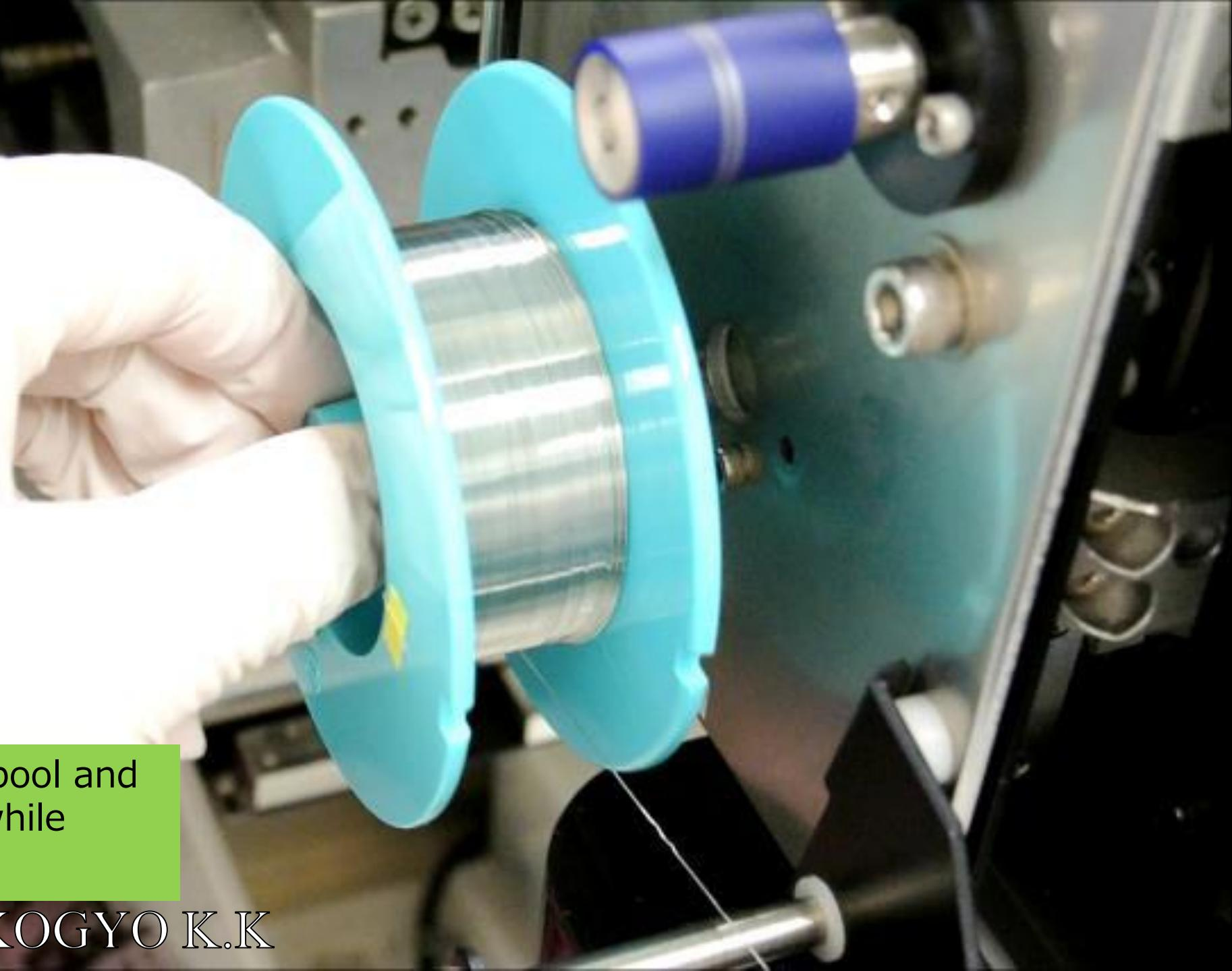
①Hold the center of the spool and remove the spool gently while holding the wire.
