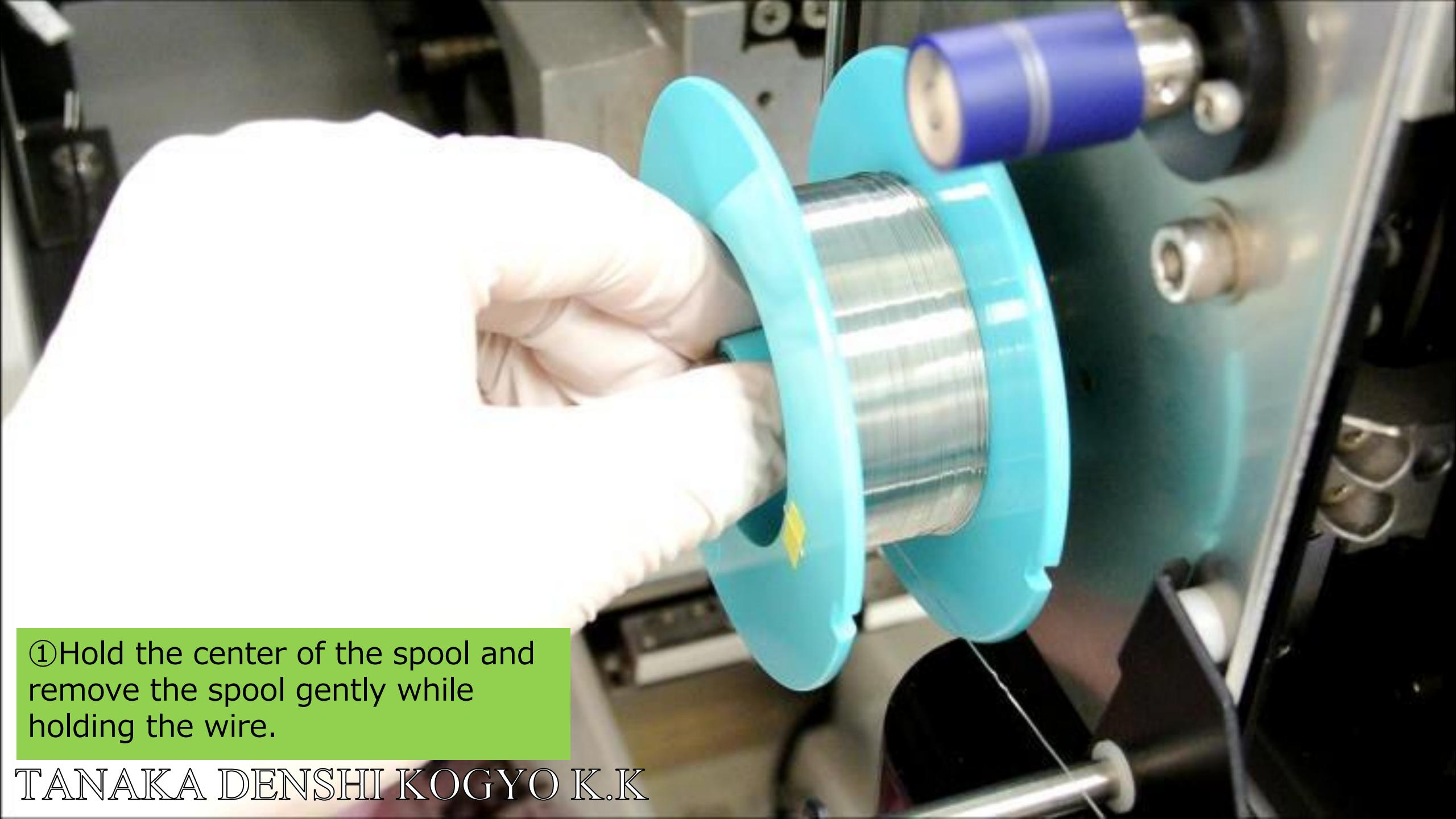
①Hold the center of the spool and remove the spool gently while holding the wire.
