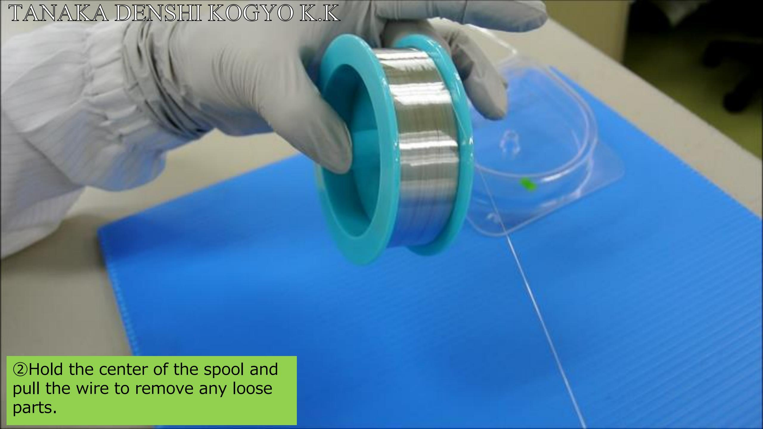
② Hold the center of the spool and pull the wire to remove any loose parts.
